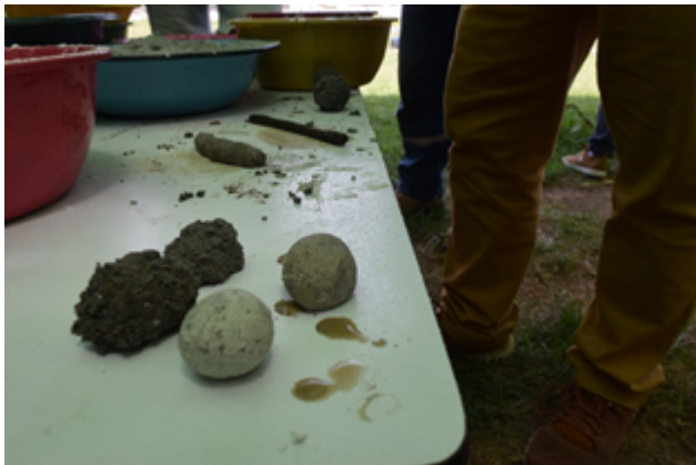
Testing with earth balls
